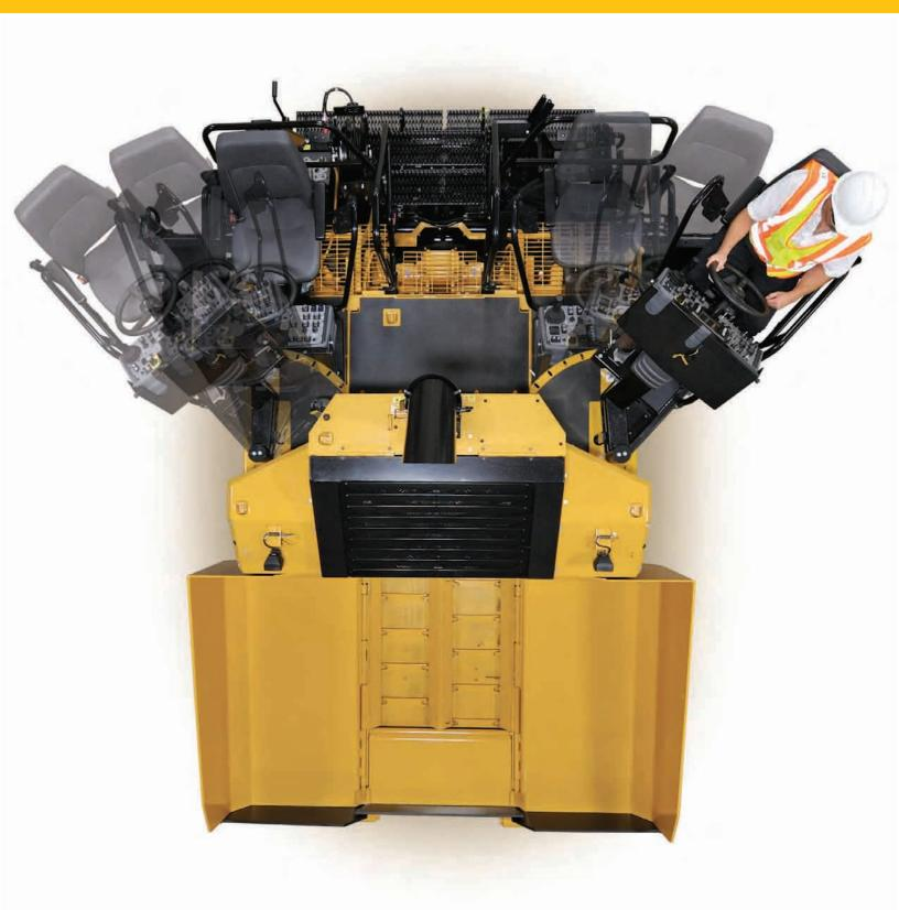
Good visibility enables effective communication that leads to smooth truck exchanges and steady material flow. Also, long hours of operation can take a toll on the crew — that's why Caterpillar designs operating stations that provide good control, visibility and comfort.
